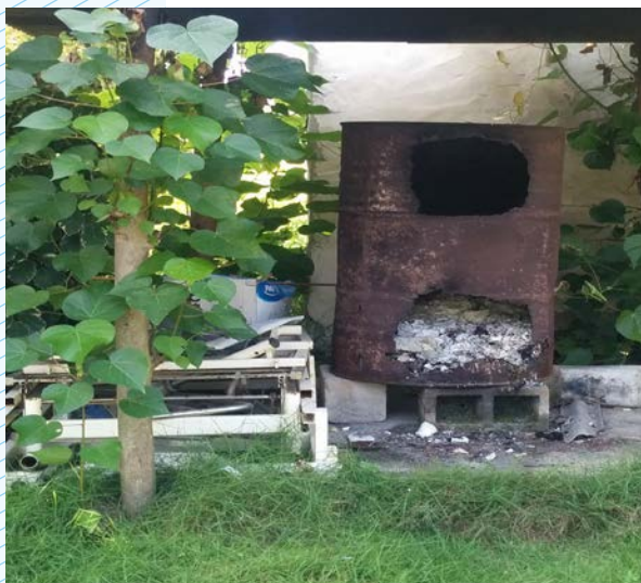
Figure 27 - Homemade incinerator at health center
